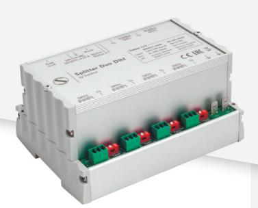
Splitter Duo DIN is special DIN rail mount device with 6 DMX input/output ports that operates as a regular splitter with 1 input and 5 outputs as well as two separated 1-to-2 splitters. All input and output channels have full galvanic isolation. Remote Device Management (RDM) compatible. The device is suitable for indoor use. Splitter is powered by 100-250 V industrial AC mains, power consumption is less than 5 watts.
