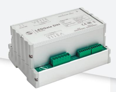
LEDGate DIN is compact LED driver with DMX512/RS-485 input. Powered from 12/24 VDC source, LEDGate is capable to control and dim 4 or 8 output lines for direct connection with LED equipment: duralight, driverless LED luminaires, etc, with independent short-circuit protection on each channel. Thanks to innovative embedded algorithms, LEDGate provides a smooth, stepless regulation in full range of intensity. With no flickering.
