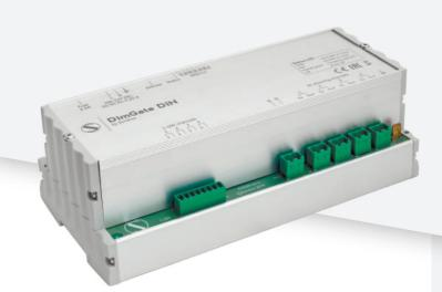
DimGate DIN is hybrid DIN-rail dimmer that converts DMX512 signal into 4 independent 110-230 VAC outputs up to 1.2 kW each to handle dimming of incandescent lamps. Additional 4 separate 1-10V (or 0-10V) outputs are supplied to integrate devices with 1-10V dimming drivers and electronic ballasts into DMX controlled surroundings.
