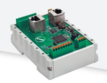
ArtNet/sACN to SPI controllers for pixel mapped indoor and outdoor LED strip installations. Two Ethernet ports and integrated switch provide cascadability. Directly convert up to 16 DMX universes into SPI to control 2,730 RGB pixels supporting 8 separate LED outputs.
