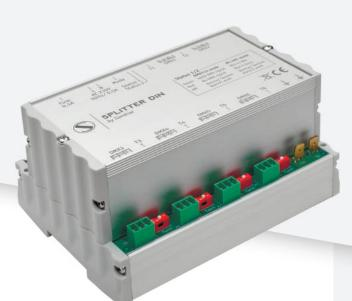
Splitter DIN DUO is special DIN rail mount device with 6 DMX input/output ports that operates as a regular splitter with 1 input and 5 outputs as well as two separated 1-to-2 splitters. All input and output channels have full galvanic isolation. Remote Device Management (RDM) compatible. The device is suitable for indoor use. Splitter is powered by 100-250 V industrial AC mains, power consumption is less than 5 watts.
