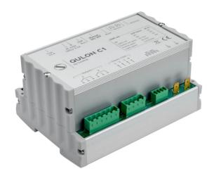
Controller QULON C1 is designed to provide remote management and diagnostics of street lighting. QULON C1 is installed into lighting power cabinet, and employs GSM/GPRS/EDGE to communicate with central QULON server. Data from the connected devices and meters are collected by QULON C1 via RS-485 interface and then sent to Qulon server via GSM/GPRS/EDGE mobile network. Programming, scheduling and troubleshooting are done remotely from QULON software.
