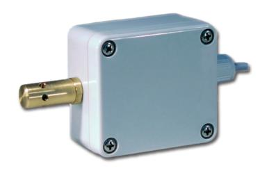
Qulon Meteo provides information about air temperature (-40°...+70°C range), relative humidity and atmospheric pressure that is useful for other telemanagement systems. Easy pole-mounting installation. Remote control and monitoring. Integrated into lighting management system. Compact and accurate as a Swiss watch.
