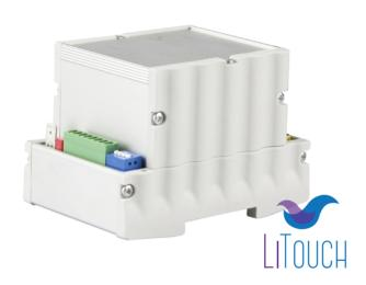
Qulon LiTouch is additional module that provides individual remote light control of luminaires with installed LiTouch nodes wirelessly via radio channel. Installed together with Qulon-C (Central Gateway) into existing lighting cabinet. Connected to the central controller Qulon-C via RS-485 interface (ModBus). Acts as a master to send/receive data to/from wireless modules (slaves). It communicates with the slaves using 800-950 MHz wireless interface.
