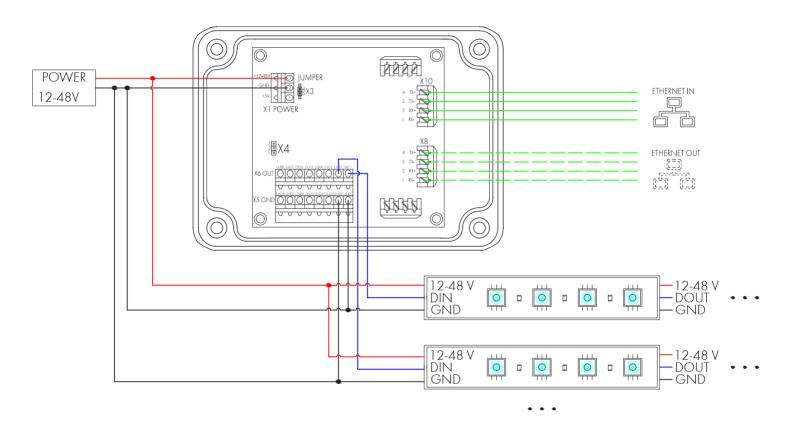
When using **12-48V** power source, set the jumper at **X3** connector. When using **5V** power source, jumper is **not** installed.
